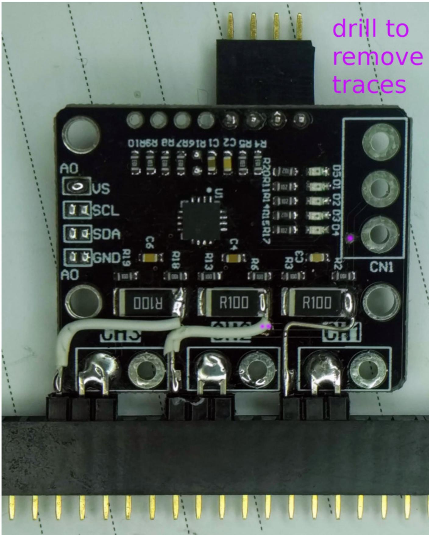
Cutting traces on both sides of board seemed like too much for me, so I decided to use hand drill to scratch top side of board at three places and disconnect ground and power input from resistors. Add three wires to connect new pin to connect load to or just connect any dupont wire to use it as 10-bit voltage adc.
