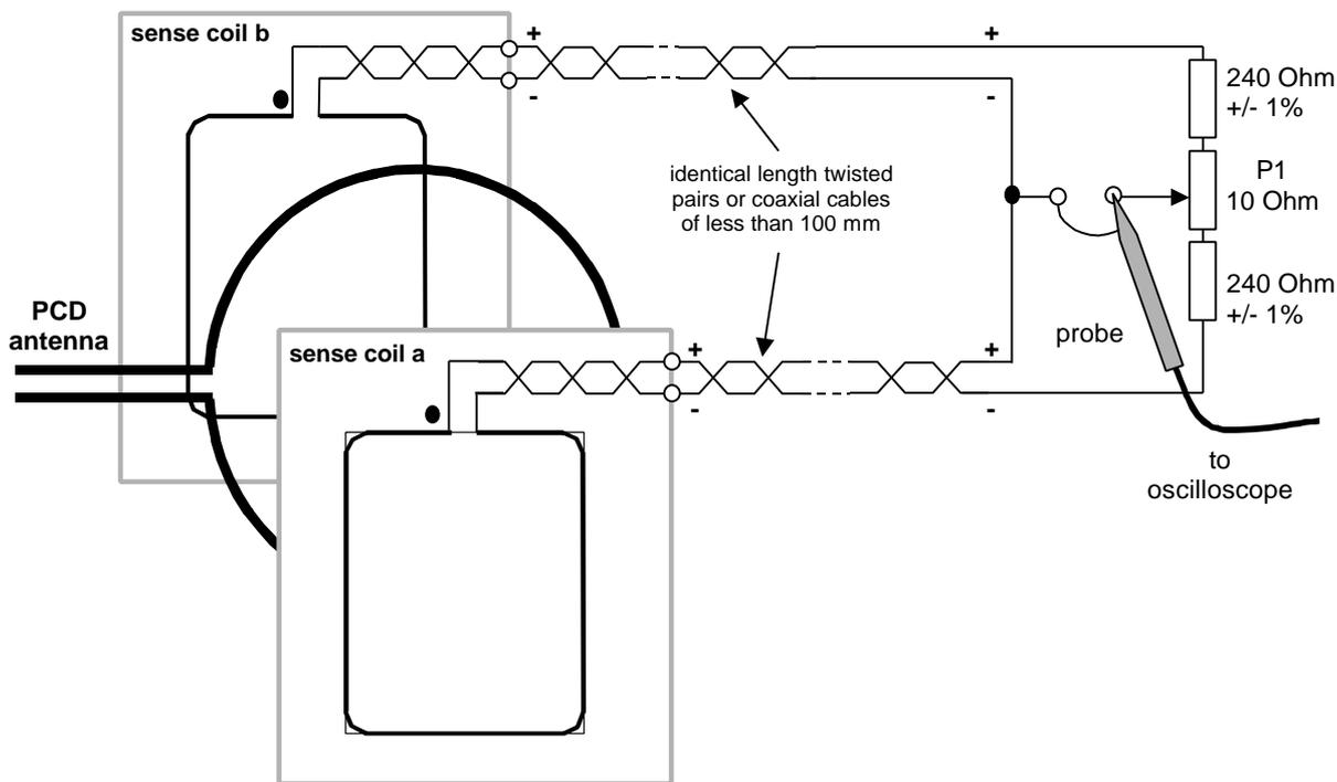
NOTE 1 In order to avoid any unintended misalignment in case of an unsymmetrical set-up the tuning range of the potentiometer P1 is only 10 Ohms. If the set-up cannot be compensated by the 10 Ohm potentiometer P1 the overall symmetry of the set-up should be checked.
